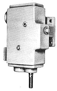
This is basically a four-way valve with the shuttle acting as the four-way spool. The movable sleeve between the shuttle and body, and the manual control spool is the control that causes reciprocation of the shuttle. The movable sleeve is operated by adjustable stop collars on the shipper rod. The manual control spool is actuated by an eccentric crank. A spring arrangement tends to hold the crank in "neutral", but it will lock in the "automatic" position and remain there until released.
