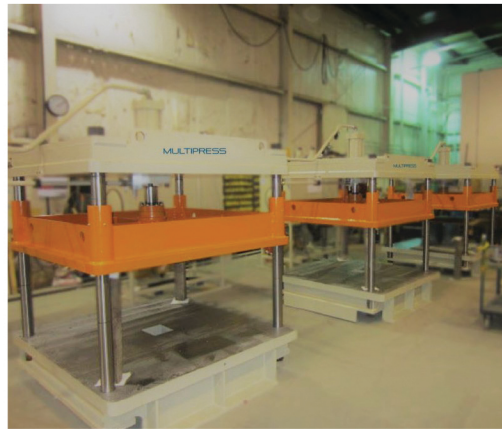
Large Platen 30-Ton Presses for transfer line
