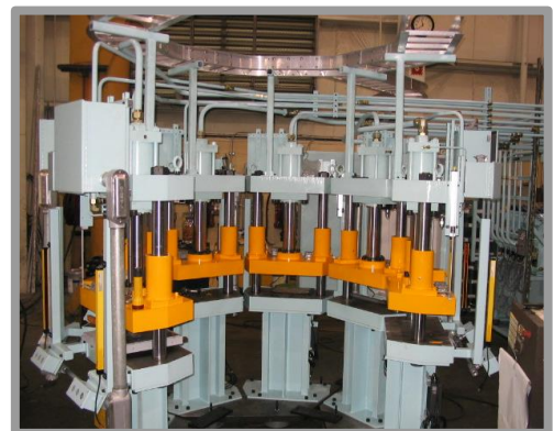
(six) 30-ton bonding presses for positioned robot loading
