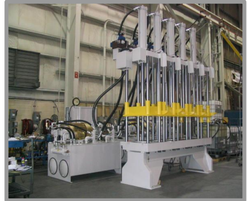
A fully rebuilt five station draw press
